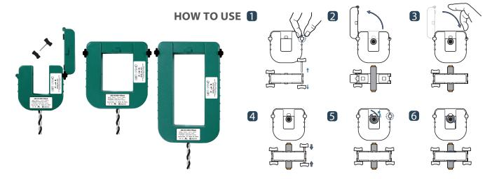
JSC series of split-core current transformer offers 100mA at secondary from sensed primary current. Without using secondary CT inside of meter, users directly connect JSC series to a meter for high accuracy metering application. It enables one meter to be adopted for various current rating by only changing primary CT so it makes compact design meter and reduces developing cost. Also, over-voltage protection circuit is included to offer safe, fast and cost effective installation.
